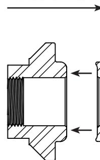
**NOTE:** The included washer is designed to contour to the shape of the included cone nut core. When installing make sure both the cone nut core and washer (if applicable) are facing the correct direction.
